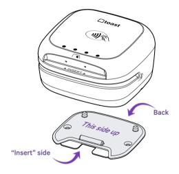
Place the reader on the plate. It can be removed if needed in the future.
